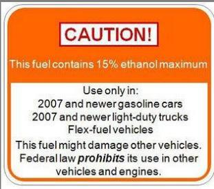
This little label on a gas pump is the only thing standing between a boater and a dangerous misfueling of his gas tanks.
