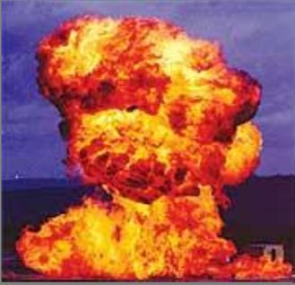
**Fig. 13 - Example of a Boiling Liquid Expanding Vapour Explosion (BLEVE)**
