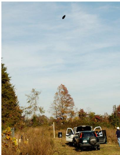
Steel drums are used for storage, transport and disposal of waste. Biological, chemical and/or radiological processes operating on drum contents may lead to an internal drum atmosphere that provides a potentially "explosive" air/fuel mixture. Given an ignition source, this mixture could subsequently result in a drum explosion or fire, most commonly referred to as drum deflagration.
